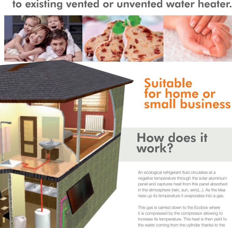
An ecological refrigerant fluid circulates at a negative temperature through the solar aluminium panel and captures heat from this panel absorbed in the atmosphere (rain, sun, wind,...). As the klea rises up its temperature it evaporates into a gas.
